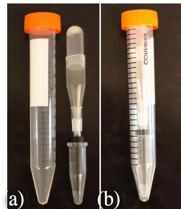
Figure C.4: Sample transfer assembly. (a) Clipped ultracentrifuge tube fits into clipped 5 mL pipette tip, which rests in 200 \mu L flame-sealed pipette tip and black funnel. The entire assembly rests in the Eppendorf tube with cap removed. (b) The assembly needs to fit inside a 15 mL orange cap tube.
