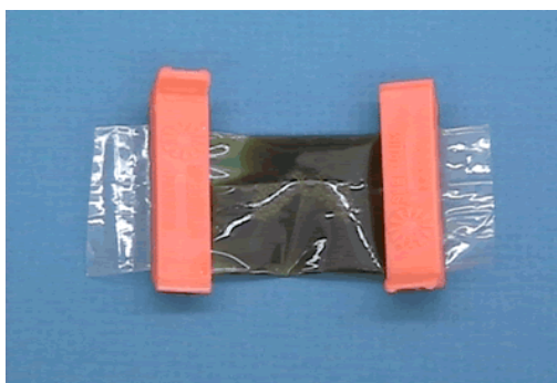
Figure C.1. Dialysis tube filled with a solution, and clipped on both ends with tube clips (4).
