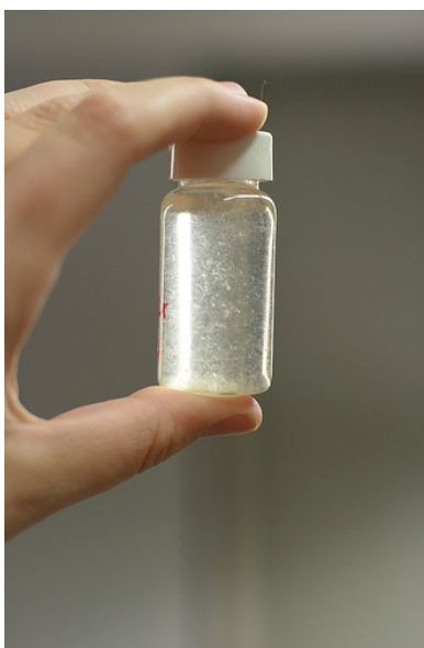
Figure A.2: Recrystallization of amt·HCl in ethyl ether and ethanol.
